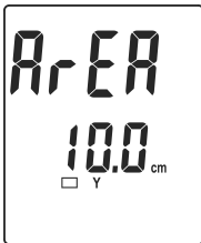
(5) Fig.5 Set Rectangle Duct Y dimension.
